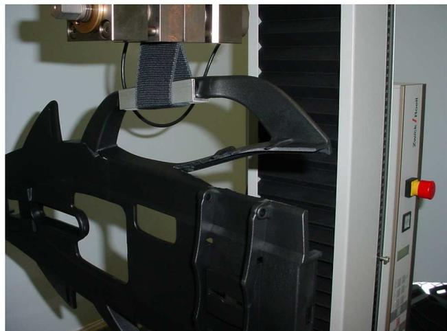
(b) After failure (ultimate tensile strength reached)
